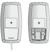
Pict. 20: Replacing batteries in the remote control (if supplied).
